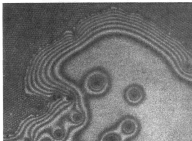
Figure 4. (Top) Interference pattern due to the slope of the liquid meniscus surrounding the ordered array (in the lower right zone). Every transition from a dark to bright band or vice versa corresponds to a 102-nm difference in the thickness of the liquid layer (low magnification). (Bottom) Interference pattern at the boundary between the ordered monolayer (the dark zone) and a "lake" (region free of particles where the substrate is covered only by a thin water layer—the bright zone) inside the array. The water layer thickness in the lake is below 50 nm, while at the boundary of the particle monolayer it is slightly below 1.7 \mu\text{m} .
