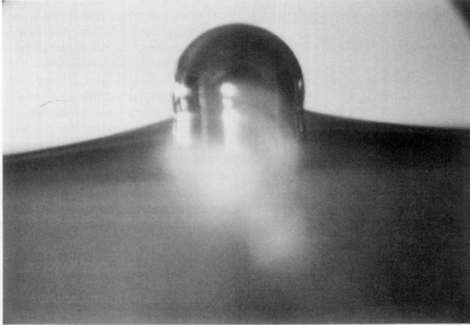
FIG. 2. Photograph of the immersed part of a mercury drop floating attached to a water-air interface. From the equatorial radius and the depth of immersion of the drop one can calculate precisely the three-phase contact angle.
