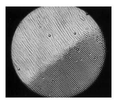
Photograph of the process of 2D array formation from latex particles, 1.7 µm in diameter, under the action of the capillary immersion force and an evaporation-driven convective flux of water (see Chapter 13); the tracks of particles moving toward the ordered phase are seen; from N.D. Denkov, O.D. Velev, P.A. Kralchevsky, I.B. Ivanov, H. Yoshimura, K. Nagayama, Langmuir 8 (1992) 3183.
