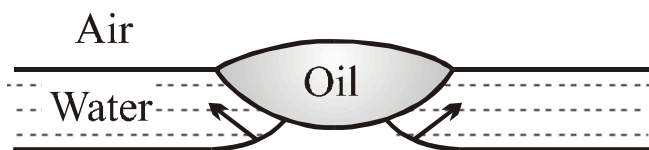
Fig. 14.15. An oil lens, initially attached to the upper film surface, enters the lower film surface. The Laplace pressure in the contact zone drives the liquid away from the lens thus dewetting its lower surface.
