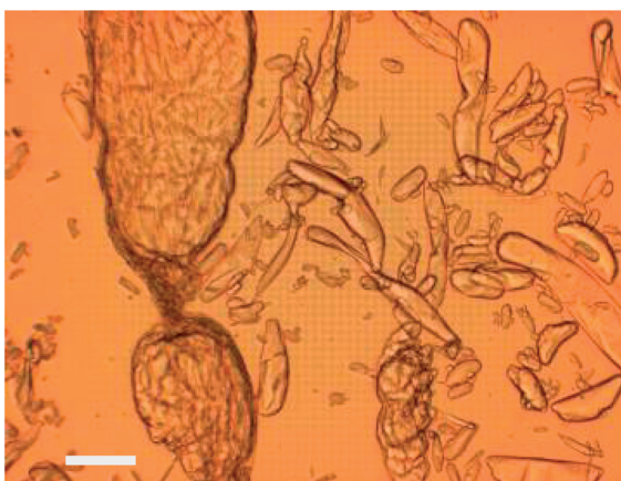
Fig. 8 Micrographs of sunflower oil-in-water emulsion droplets, stabilized by (A) BSC and (B) QD saponins. The droplets have wrinkled surfaces and many are with non-spherical, elongated shape that does not relax for many days, which is indicative for the formation of an elastic adsorption layer with unusual rheological properties at the oil-water interface. The scale bar in the image is 20 \mu\text{m} .
