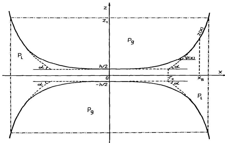
Fig. 1. The transition between a thin liquid film and the capillary meniscus is smooth. The solid and dashed lines represent the real and the extrapolated interfaces, respectively.
