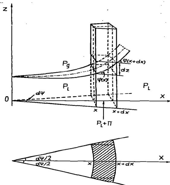
Fig. 2. A volume element in the transition region used for deriving the conditions for local mechanical equilibrium.
